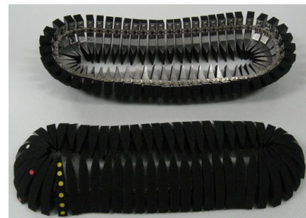
Fig.8: Belt of the Crawler (top one is reverse side of the crawler)
